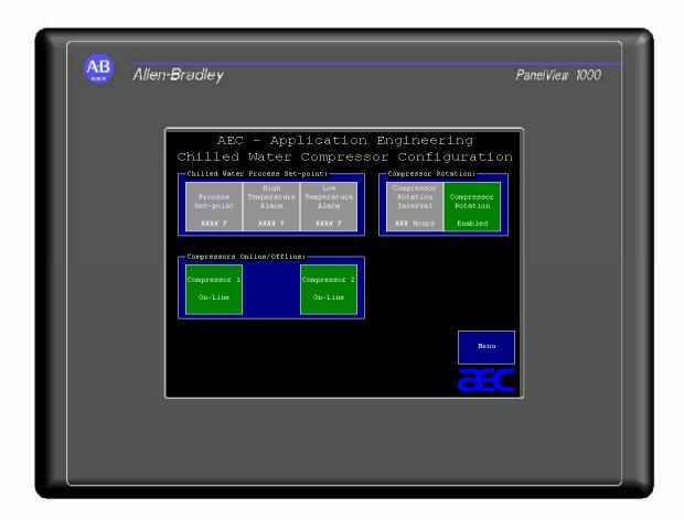
■ Touch the screen corresponding with the compressor you want to bring On-Line or Off-Line. The background color of the square turns green for On-Line and black for Off-line.
